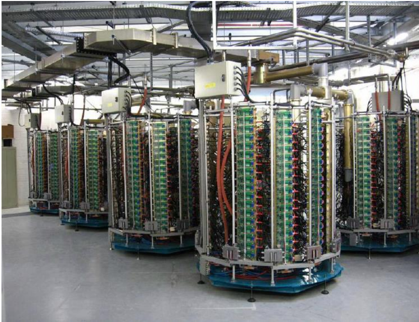
SOLEIL 45 kW @ 352 MHz tower solid state amplifiers (2004 & 2007)
