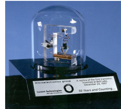
First transistor invented at BELL labs in 1947
